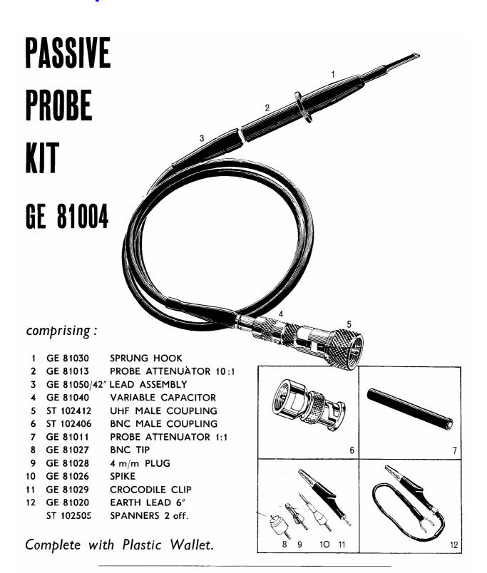
This Probe Kit is for use with instruments having an input resistance of 1 Megohm and capacities of 15-55 pf. Additional mating couplings are available with TNC, N or C interfaces as extras. Variations are also available to order for instruments having different input resistances and/or capacities.
